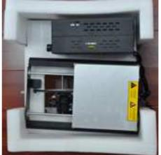
5. Put the Base onto a table or floor. Never drag the black cable.
