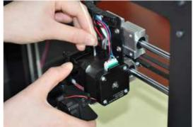
4.4 Navigate to Extruder—Extr.position. Turn the buttom clock wise to load the filament.
