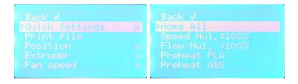
Navigate to **Quick setting---Disable stepper**. Then there's no power on every motor. So you are able to move the extruder on X axis freely. And the printing platform can move on Y axis freely too. By hand move the extruder to different positions over the build platform, while adjusting the spacing between the extruder nozzle and platform with the knobs under the platform and a sheet of paper placed between the platform and nozzle.
