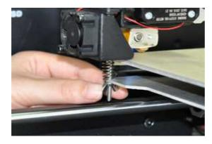
• The distance between the extruder nozzle and the build plate should be about the thickness of the A4 paper. It's about .12 mm thick, and should work great. If you haven't got the Support card on hand, a sticky note works well, too.
